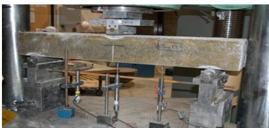
Fig; 7.3 Beam test setup under quasi-static loading
