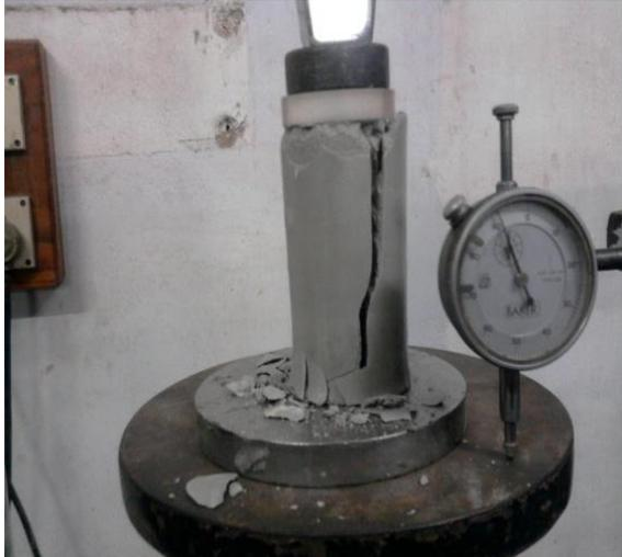
Fig.4.1. Failure model in UCS.
