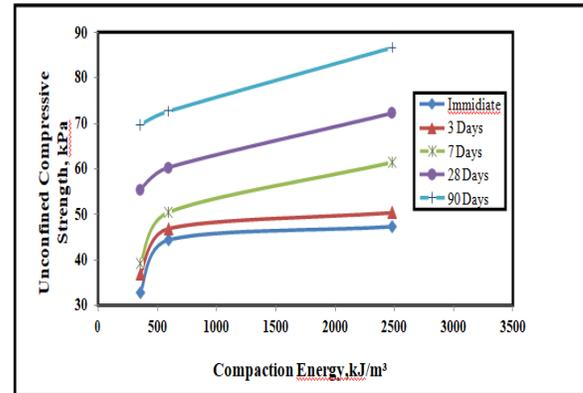
Fig.4.2. Variation of Unconfined compressive strength with Compactive energy at different curing period
