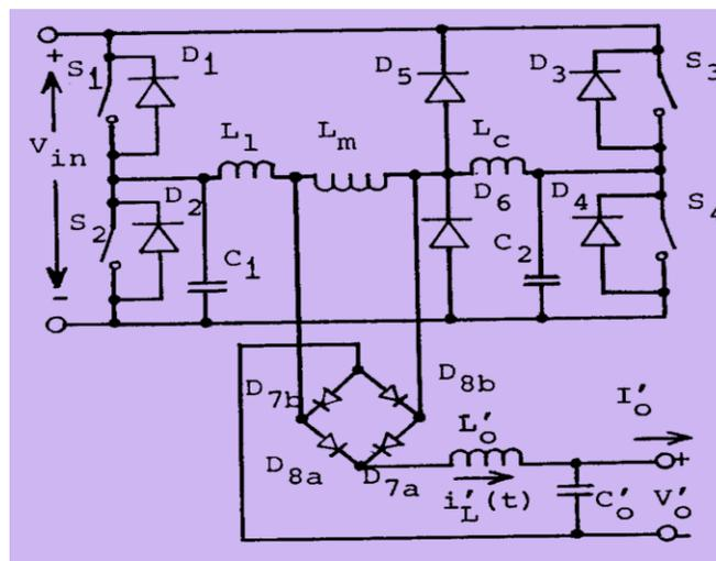
**Figure 2: The equivalent circuit of the converter**
