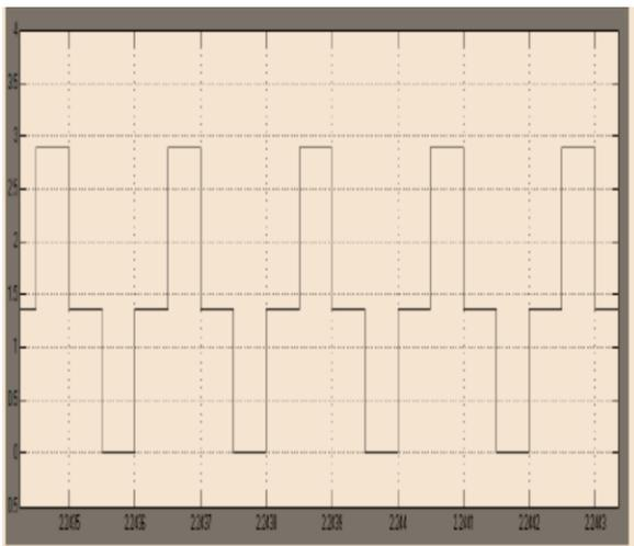
Figure: 8 Current  $i_{ds}$  of switch  $M_4$
