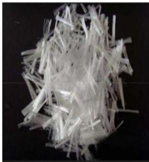
Figure 3: Polypropylene fiber
