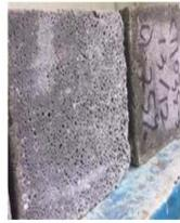
Figure 2: Foam concrete
