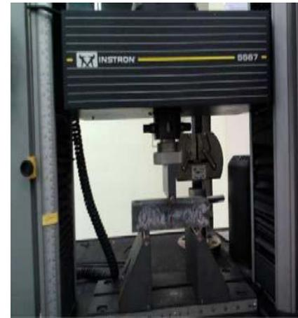
Figure 5: Setup for flexural test
