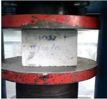
Figure 4: Setup for compression test
