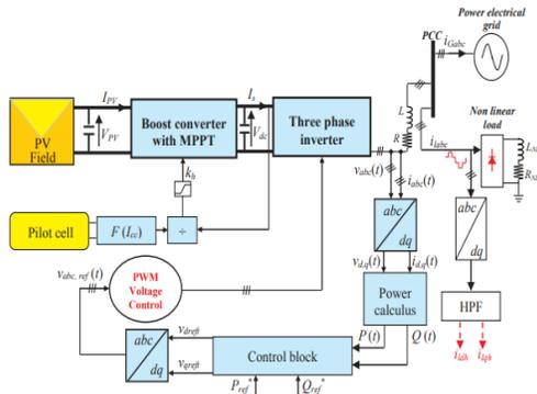
Fig. 5. Control scheme of the PWM inverter for power generation and harmonic mitigation.
