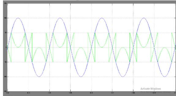
Fig: Fundamental and harmonic components of  $i_{la}$  (A).
