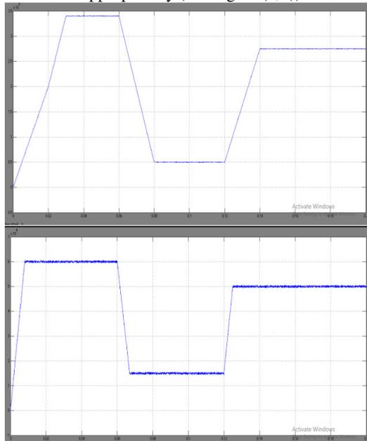
Fig8: Simulation results of a decoupled power control of the PVS: (a) Active and reactive powers in (kW) and (kVAr) respectively
