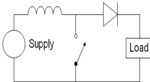
Fig.2 The basic schematic of a boost converter
