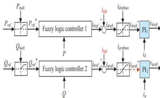
Fig. 6. Control block of the PWM inverter.
