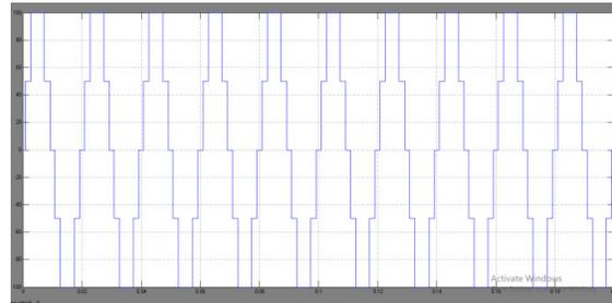
Fig10: Characteristics of the studied non linear load: Phase current component  $i_{la}$
