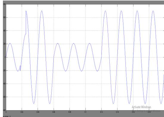
Fig9: Phase current  $i_a$  (A) at the output of the inverter.
