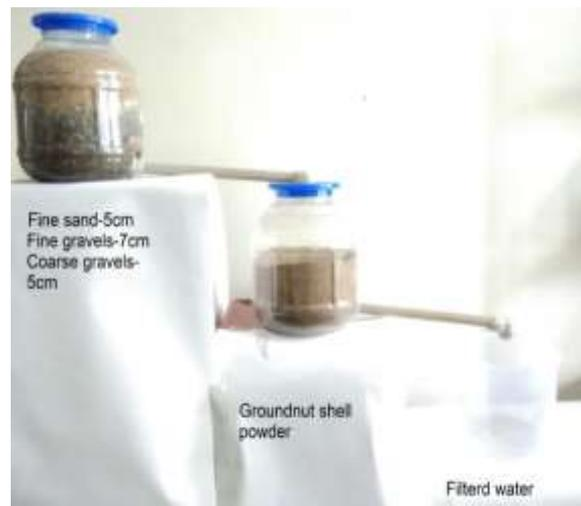
**Fig 2.** Set Up Of Filtration Of Groundnut Shell Powder
