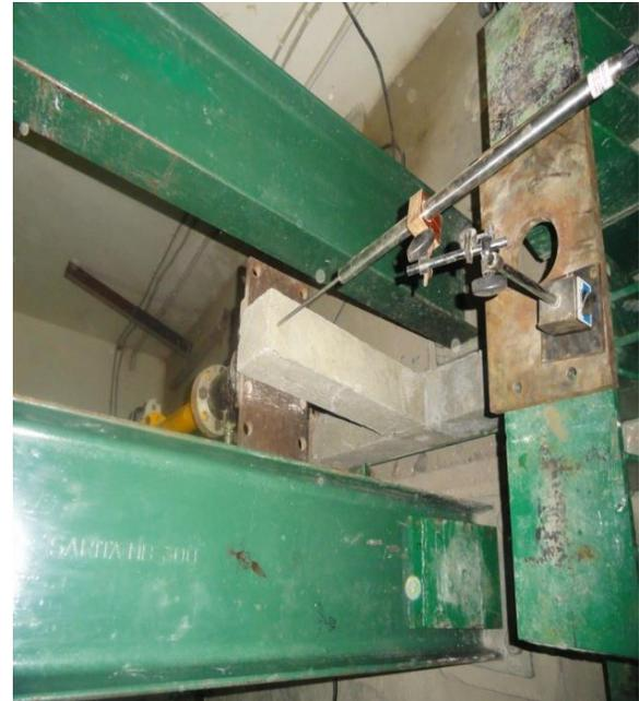
Fig. 8. Testing on Beam-Column joint
