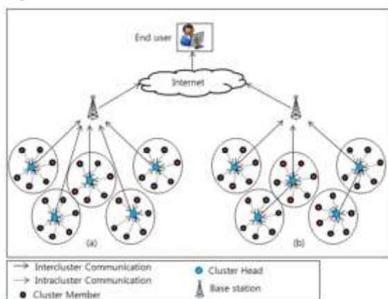
**Figure 2.** Cluster-based wireless sensor network (WSN) with different data communication scenarios: (a) single-hop communication and (b) multi-hop communication from sensor nodes to the end user through base station (BS).
