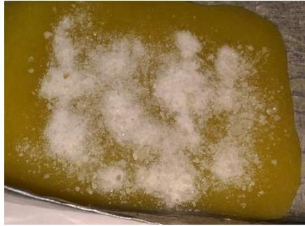
**Fig.5. Aluminium oxide nanoparticles on Epoxy layer**
