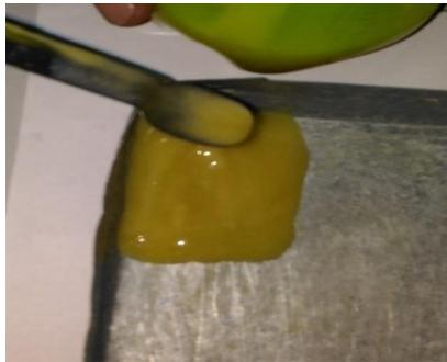
**Fig.4.Forming epoxy layers**
