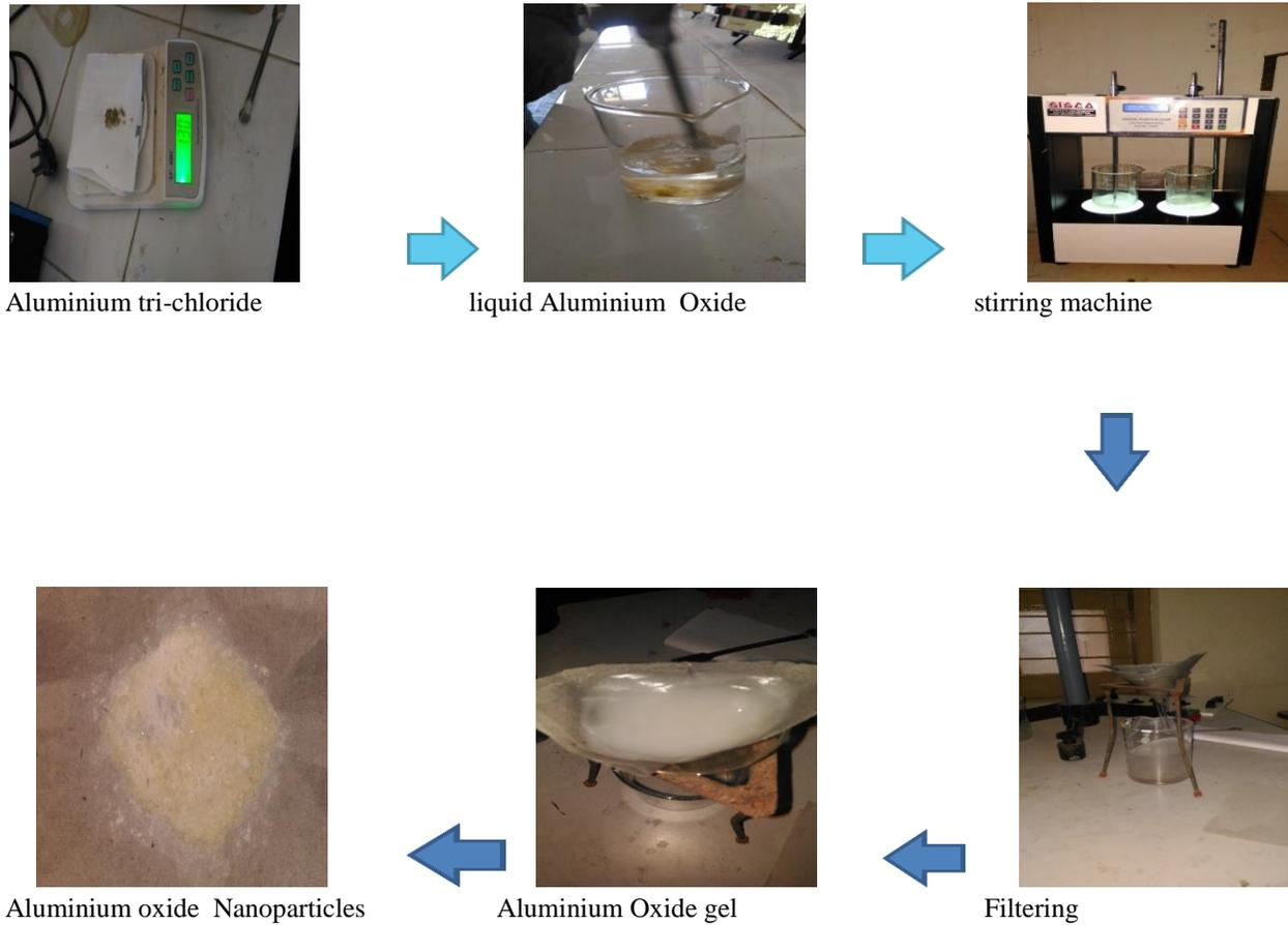
Figure1. show the Aluminium oxide nanoparticles. These particles were synthesized by sol-gel technique. The precursor material used here is Aluminium tri-chloride (AlCl<sub>3</sub>). Ethanol and Ammonia used as solvent and catalyst respectively.
