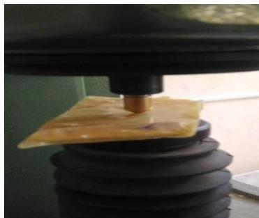
Fig 8. Rockwell Hardness testing machine
