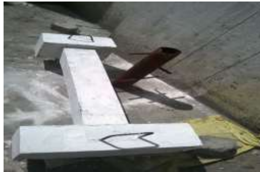
FIG:4 RC Column Specimen
