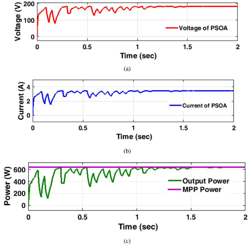
Figure 7. Simulation results for PSOA. (a) Voltage (b) Current (c) Output power vs MPP power
