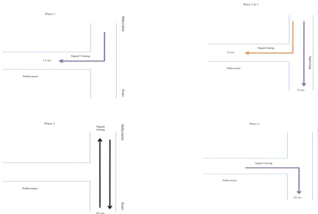
Figure 2. Details of Signal Phase Timings
