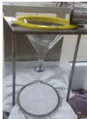
Figure 8. Analysis of water repellent finish
