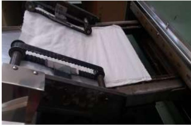
Figure 4. Drying of fabric in stenter machine.
