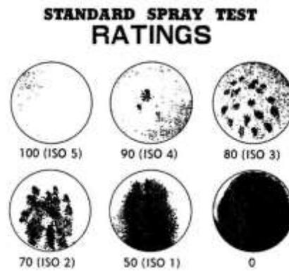
Figure 6. Average table of textile water repellent ratings
