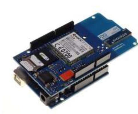
Figure 4. GSM Module with dedicated SIM Slot
