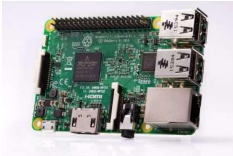
Figure 2. Raspberry Pi Module 3 Model B
