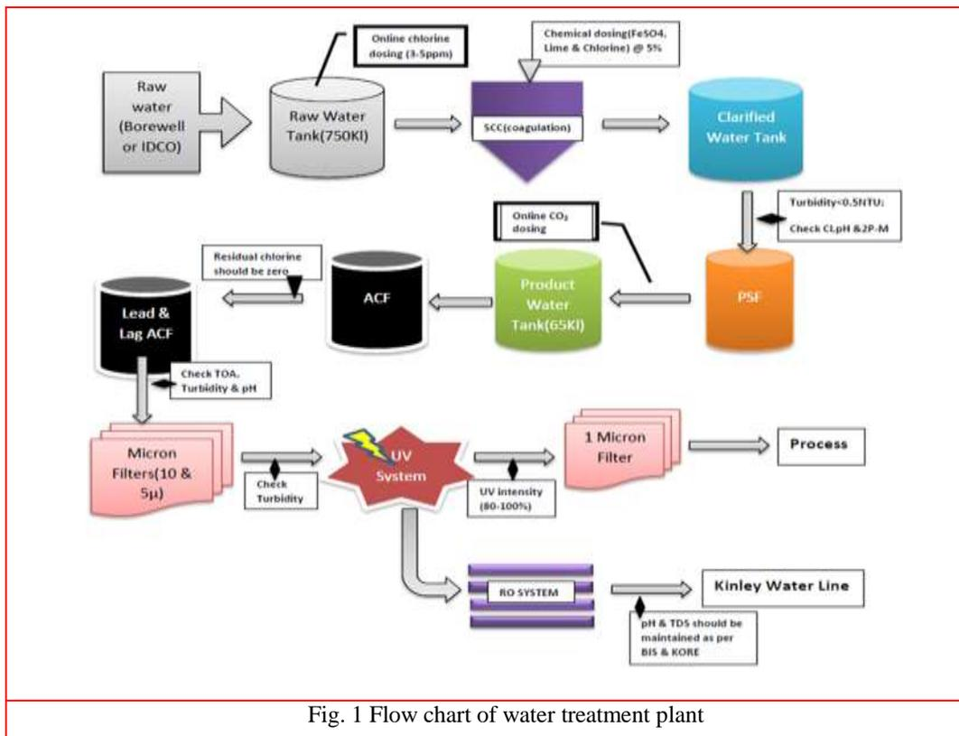
Fig. 1 Flow chart of water treatment plant
