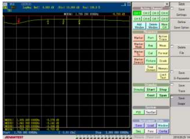
Fig. 24. Measurement result for input return loss ( S_{11} ) of implemented LNA
