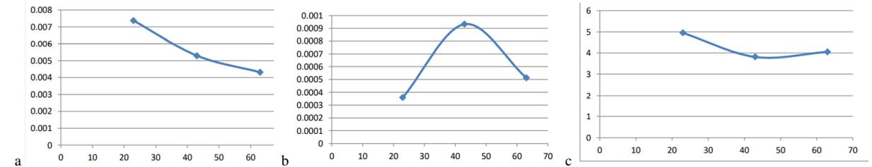
Figure 4. The electrode used is Aluminium and a graph is drawn by taking input current on x axis with (a) MRR (b) TWR (c) Surface roughness
