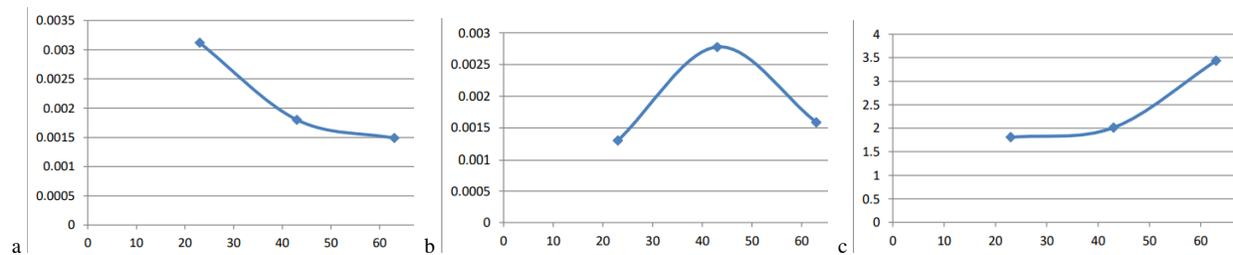
Figure 5. The electrode used is Bronze and a graph is drawn by taking input current on x axis with (a) MRR (b) TWR (c) Surface roughness
