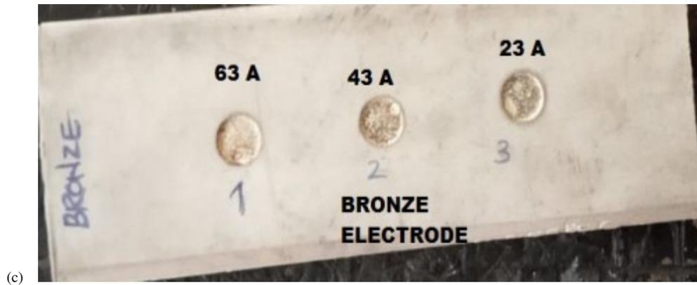
Figure 2. Samples of the work piece with electrode material of (a) Copper(b) Aluminium (c) Bronze
