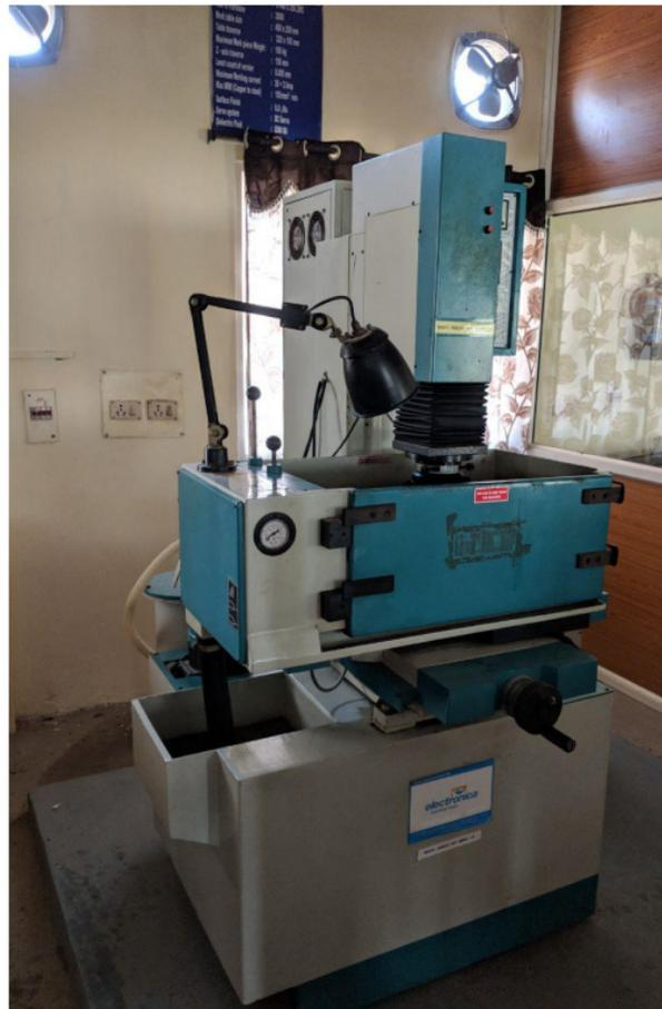
Figure 1. ElectronicaC-425 EDM machine used for experimentation
