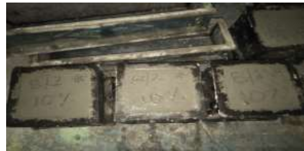
Fig.6. Casting of Specimen
