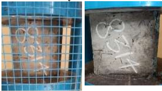
Fig8. 14 th day test a) before test b) after test
