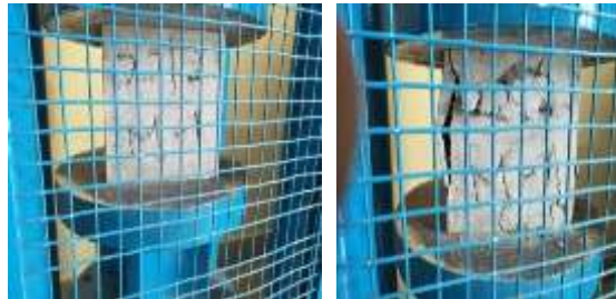
Fig 9. 28 th day test a) before test b) after test
