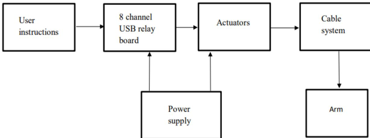
Figure 5.1 Block Diagram of Octacle Arm
