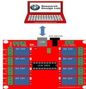
Figure 4.1 USB 8 Channel Relay Board to PC connection
