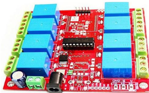
Figure 2.7 RDL 8 Channel Relay Board
