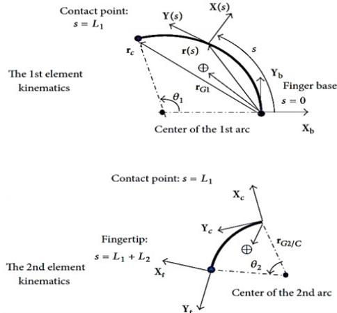
Figure 5.2 Backbone Kinematics
