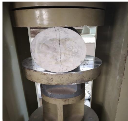
Figure 4. Split Tensile Test
