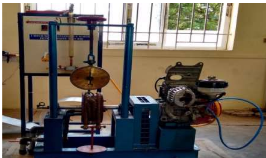
Figure.1 Experimental setup of SI Engine
