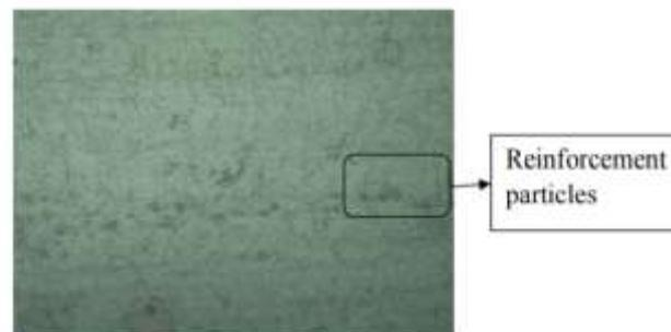
Fig.3.3.1b. Microstructure of Al-5% Cu (500X)
