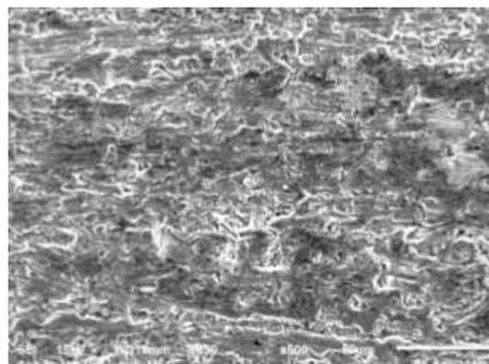
Figure.3.4.1a. SEM photograph of AL-5%Cu (500X)
