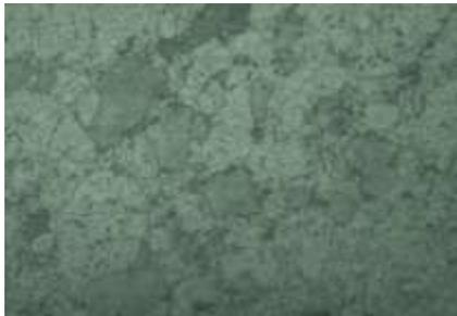
Figure.3.3.1f. Microstructure of Al-15%Cu (500X)
