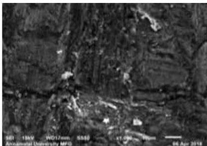
Figure.3.4.1d SEM photograph of AL-10%Cu (1000X)
