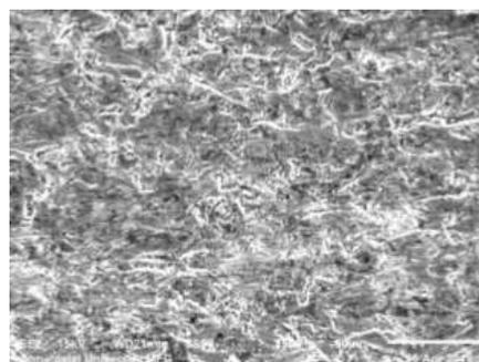
Figure.3.4.1e SEM photograph of AL-15%Cu (500X)
