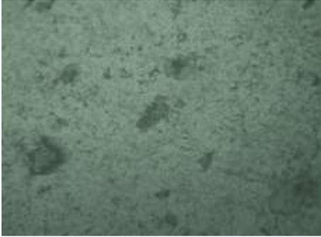
Figure.3.3.1d. Microstructure of Al-10%Cu (500X)
