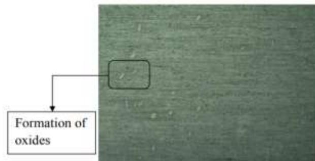
Fig.3.3.1a. Microstructure of Al-5% Cu (100X)
