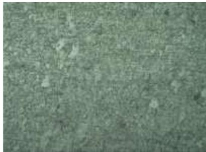
Figure.3.3.1e. Microstructure of Al-15%Cu (100X)
