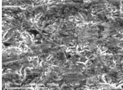
Figure.3.4.1f SEM photograph of AL-15%Cu (1000X)
