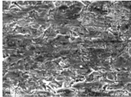
Figure.3.4.1b.SEM photograph of AL-5%Cu (1000X)
