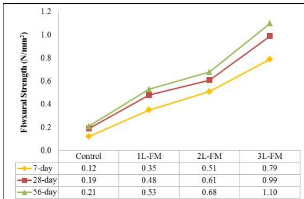
Figure 7. Flexural strength of foamed concrete of 600kg/m<sup>3</sup> with different layers of jacketing
