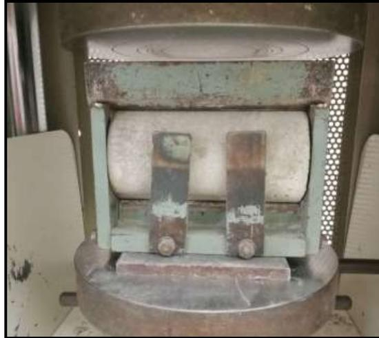
Figure 4. Setup for splitting tensile test in accordance to ASTM C496
