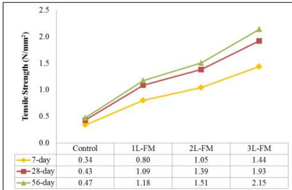
Figure 10. Splitting tensile strength of foamed concrete of 1200kg/m<sup>3</sup> with different layers of jacketing
