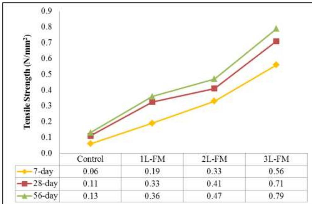
Figure 9. Splitting tensile strength of foamed concrete of 600kg/m<sup>3</sup> with different layers of jacketing
