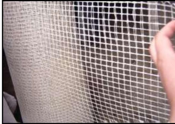
Figure 1. Fibermesh of 160gsm used in this research
