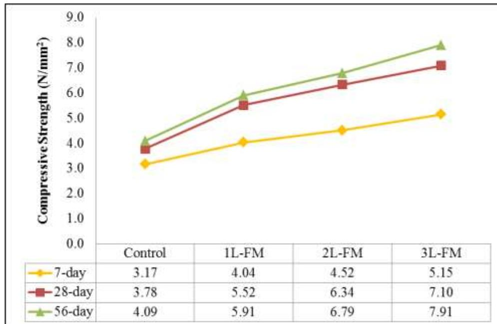
Figure 6. Compressive strength of foamed concrete of 1200kg/m<sup>3</sup> with different layers of jacketing
