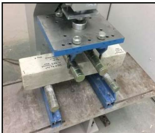
Figure 3. Setup for 2-point bending test according to BS-EN 1521
