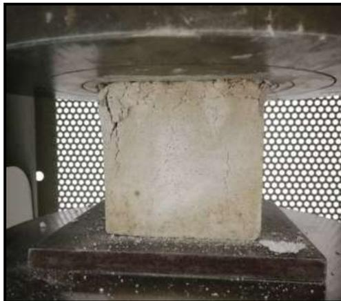
Figure 2. Setup for compression test according to BS-EN 12390
