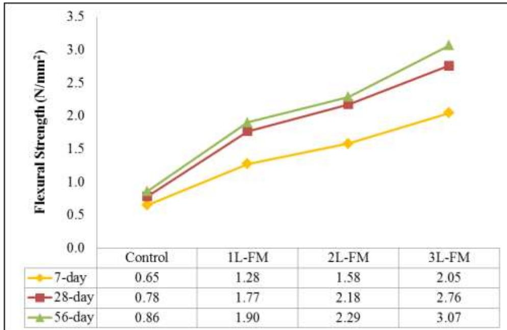
Figure 8. Flexural strength of foamed concrete of 1200kg/m<sup>3</sup> with different layers of jacketing
