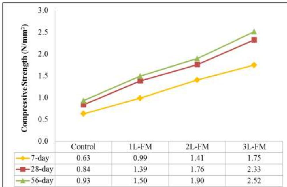
Figure 5. Compressive strength of foamed concrete of 600kg/m<sup>3</sup> with different layers of jacketing
