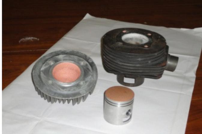
Figure 1 Photographic view of copper coated piston, liner and copper coated cylinder head
