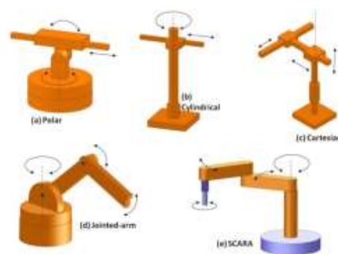
Figure 1 A) Polar, B) Cylindrical, C) Cartesian, D) Jointed-Arm, E) SCARA
