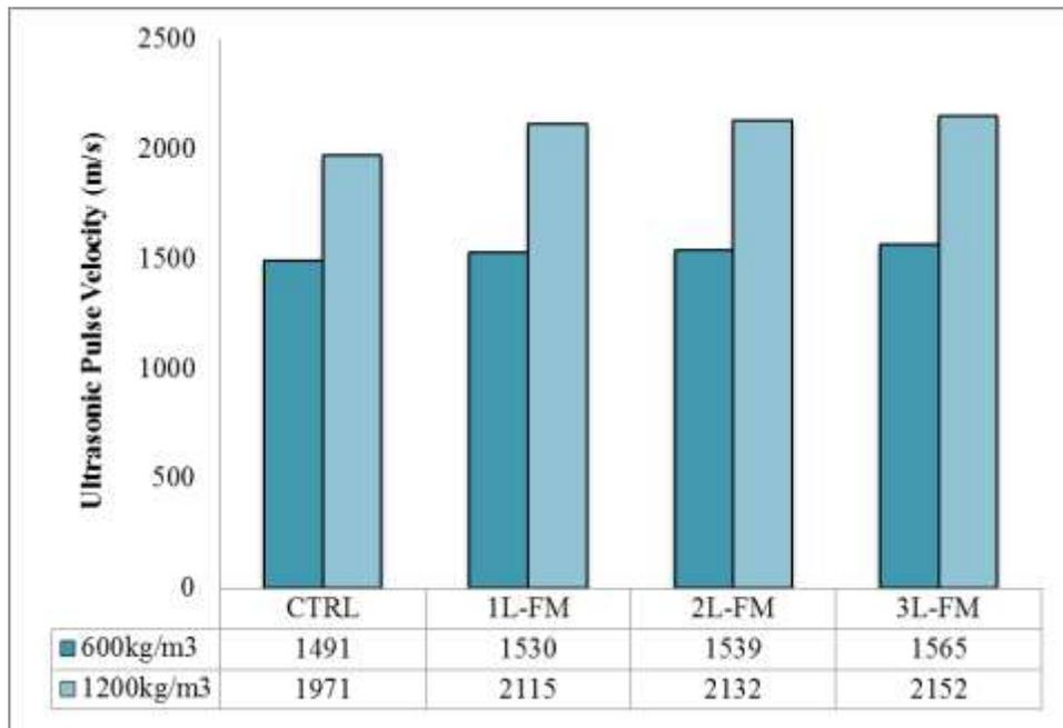
Figure 3. Ultrasonic Pulse Velocity of foamed concrete with different layers of fibermesh confinement
