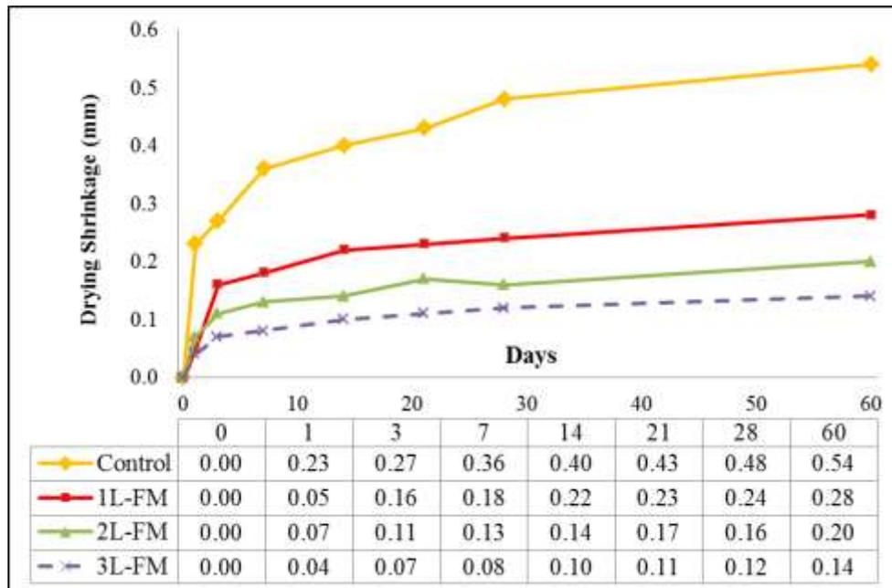
Figure 5. Drying shrinkage of foamed concrete of 1200kg/m<sup>3</sup> density with different layers of fibermesh confinement
