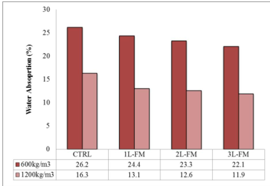
Figure 2. Water Absorption of foamed concrete with different layers of fibermesh confinement
