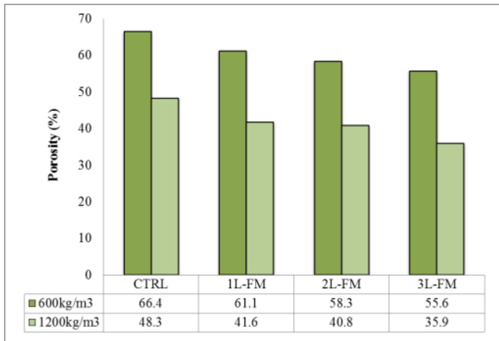
Figure 1. Porosity of foamed concrete with different layers of fibermesh confinement
