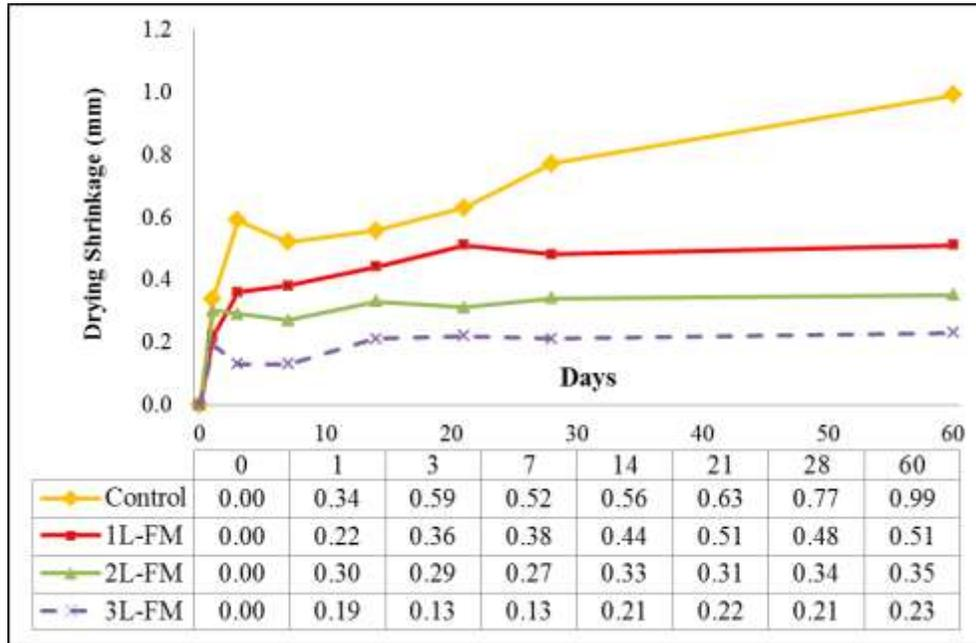
Figure 4. Drying shrinkage of foamed concrete of 600kg/m<sup>3</sup> density with different layers of fibermesh confinement
