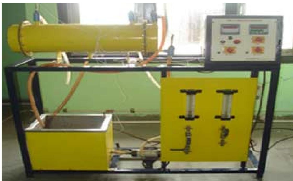
Fig.1: Experimental set up of heat exchanger
