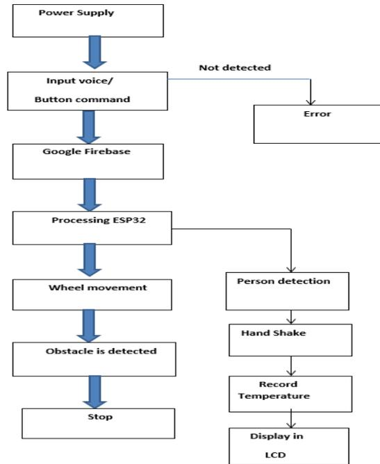
Figure 1. Working Algorithm of Humanoid
