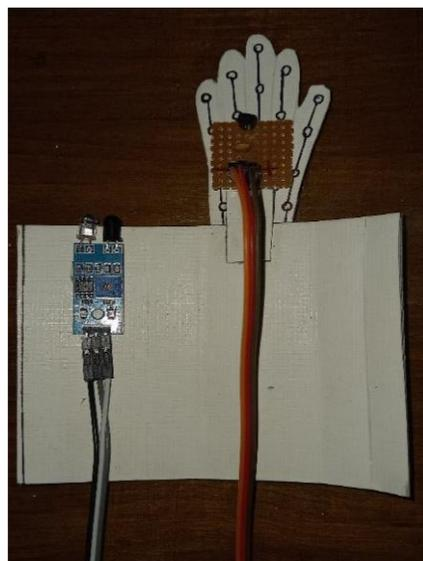
Figure 4. Servo Controlled hands with temperature sensor
