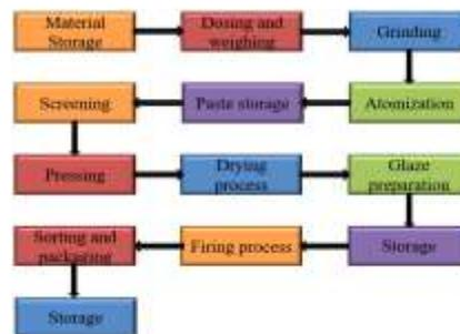
Figure 1. Description of the ceramic processing
