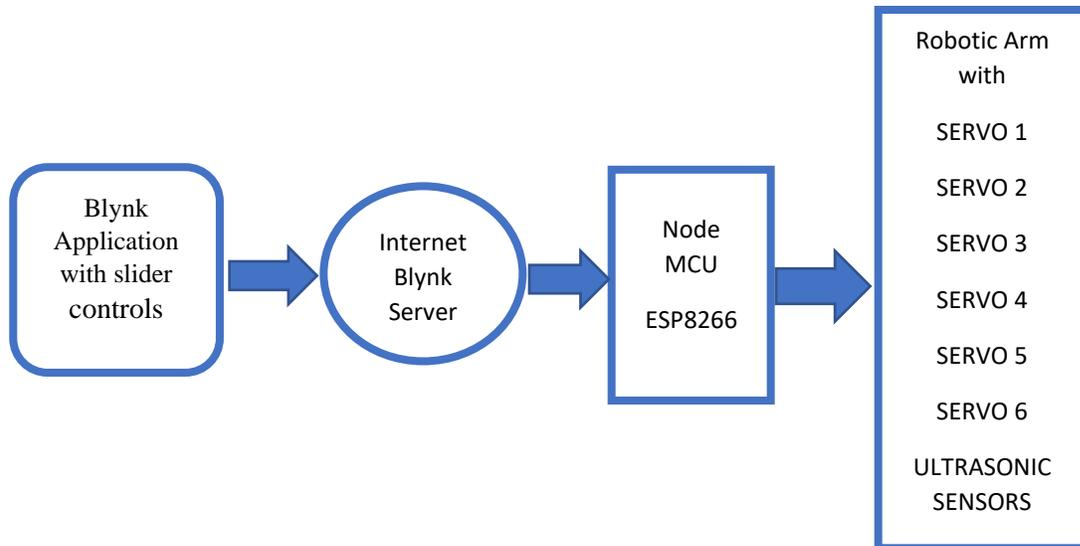
Figure 3: Functionality Of IOT based Smart Robotic Arm
