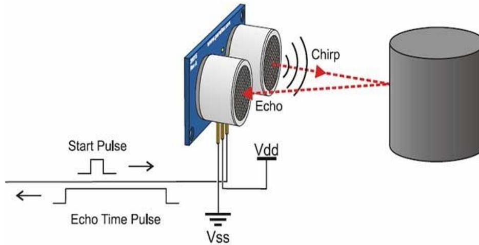
Figure 1: Working of Ultrasonic sensor
