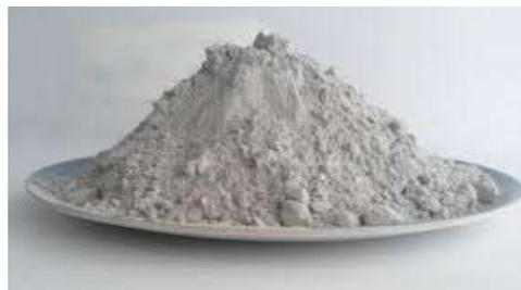
Figure 2.2 Ground granulated blast furnace slag(GGBS)
