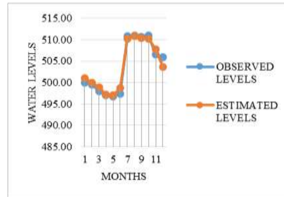
Fig. 21. Comparative analysis for Well No.5 by SCG algorithm
