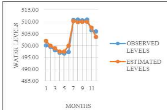
Fig. 20. Comparative analysis for Well No.5 by LM algorithm
