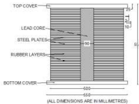
Figure 8: Schematic Diagram of LRB
