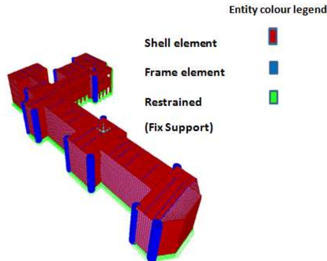
Figure 3: 3D View of Model
