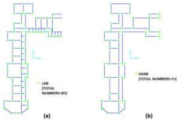
Figure 10: Beams At Plinth Level and Position of Bearings (a) LRBs (b) HDRBs
