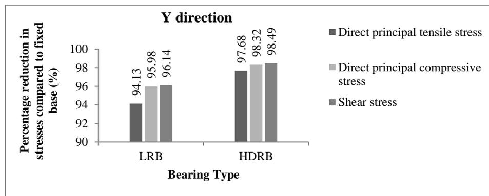
Figure 16: Percentage reduction in stresses compared to fixed base in Y direction
