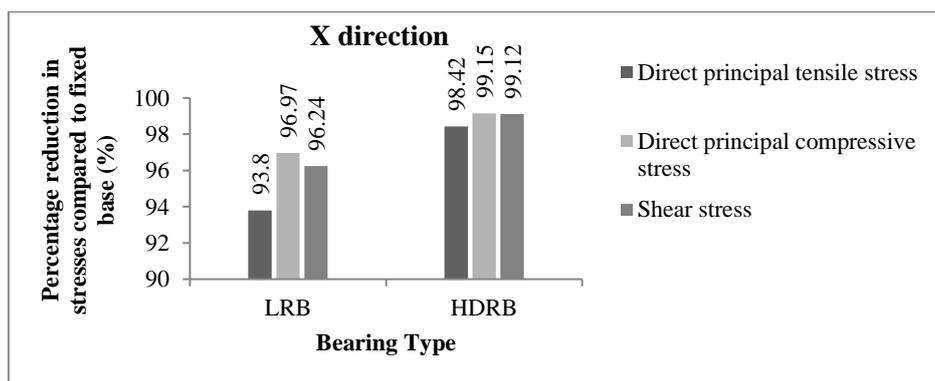
Figure 15: Percentage reduction in stresses compared to fixed base in X direction
