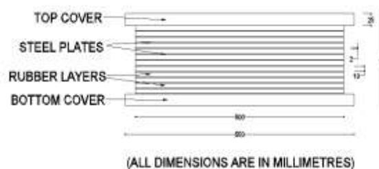
Figure 9: Schematic Diagram of HDRB
