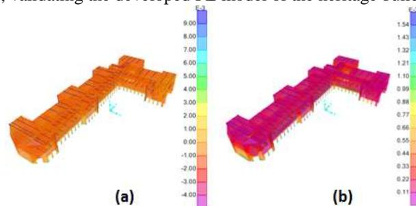
Figure 4: (a) Direct Principal Stresses (b) Shear Stress Under Gravity Load.
