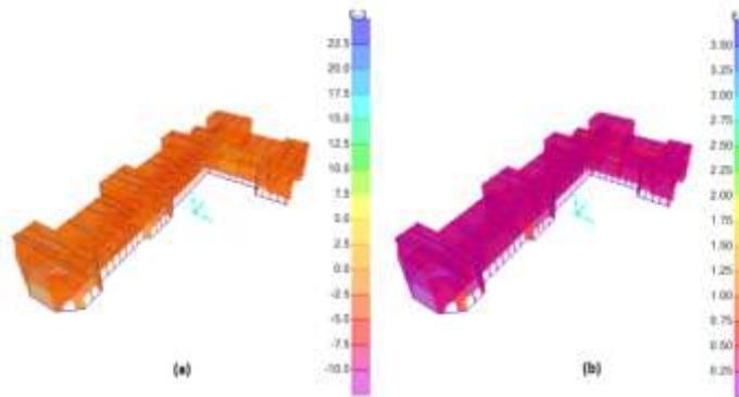
Figure 13: (a) Direct Principal Stresses in X Direction (b) Shear Stress in X Direction for HDRB.
