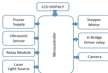
Figure 1: A schematic layout of controller element
