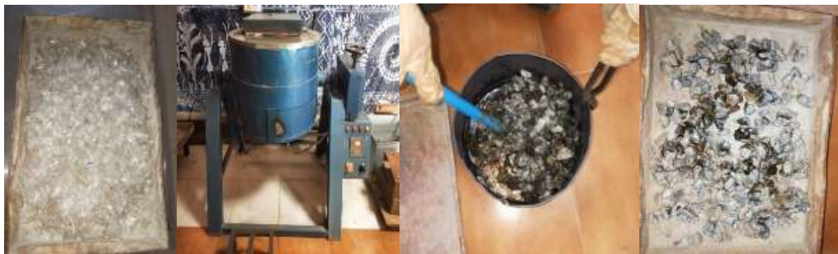
Fig 2: (A) Shredded PET (B) Furnace (C) Coating of melted PET on aggregate (D) Plastic Coated Aggregate
