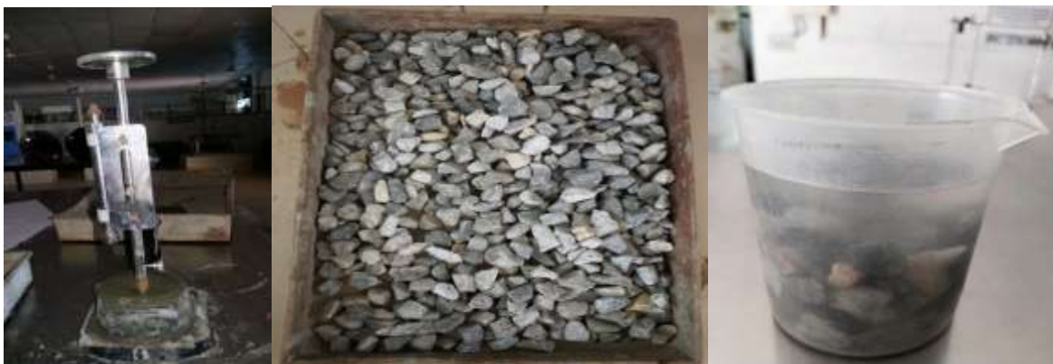
Fig 1: (A) Setting time of cement (B) Graded aggregates (C)Water absorption of aggregate
