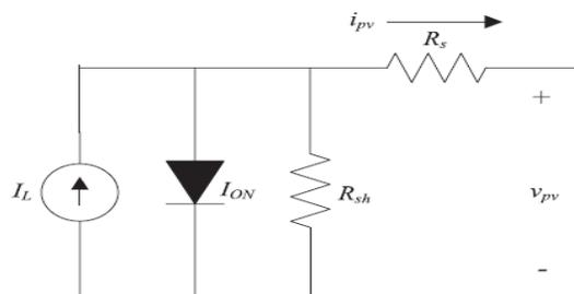
Fig.1 Equivalent circuit diagram of the PV cell
