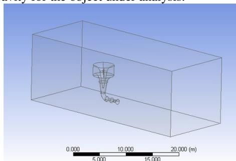
Figure 4. Computational fluid domain around the involox
