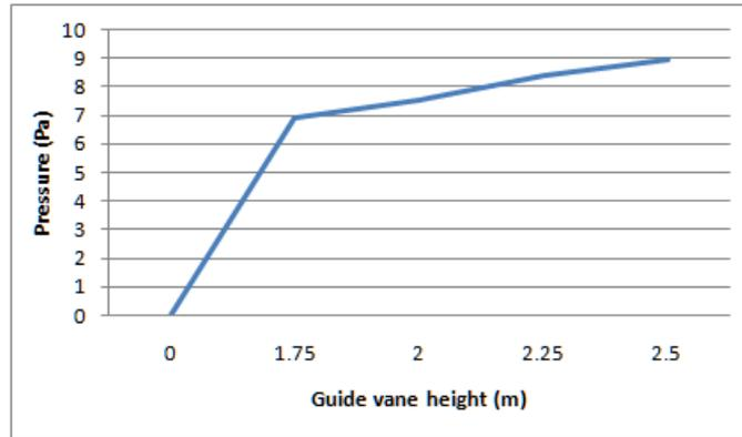
Figure 9. Variation of static pressure with guide vane height
