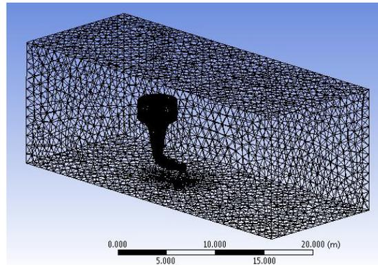
Figure 5. Meshed model of invelox duct
