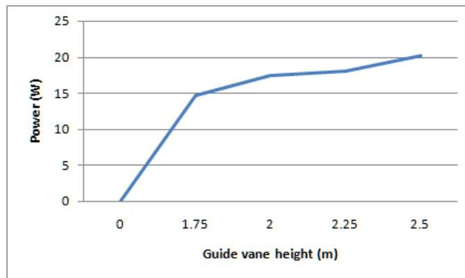
Figure 10. Variation of power produced by turbine with guide vane height
