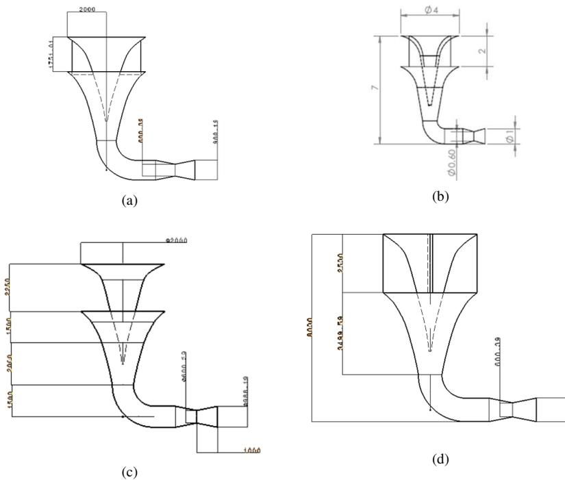
Figure 2. Geometry of involox ducts with 4 different guide vane heights
