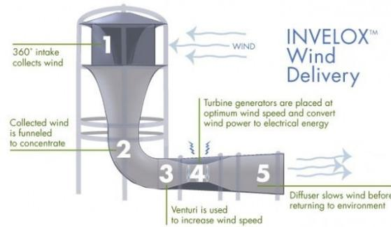
Figure 1. Schematic of the INVELOX wind delivery system (Source: Wind fair)
