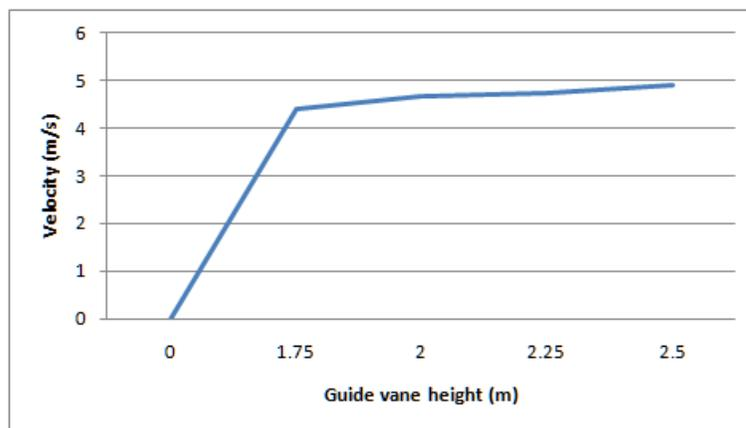
Figure 8. Variation of velocity with guide vane height
