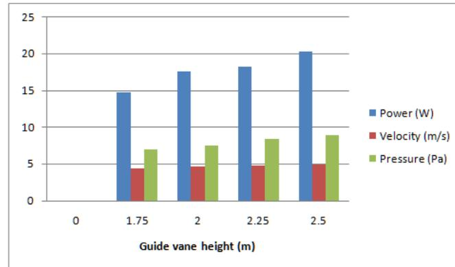
Figure 11. Comparision of parameters with guide vane height
