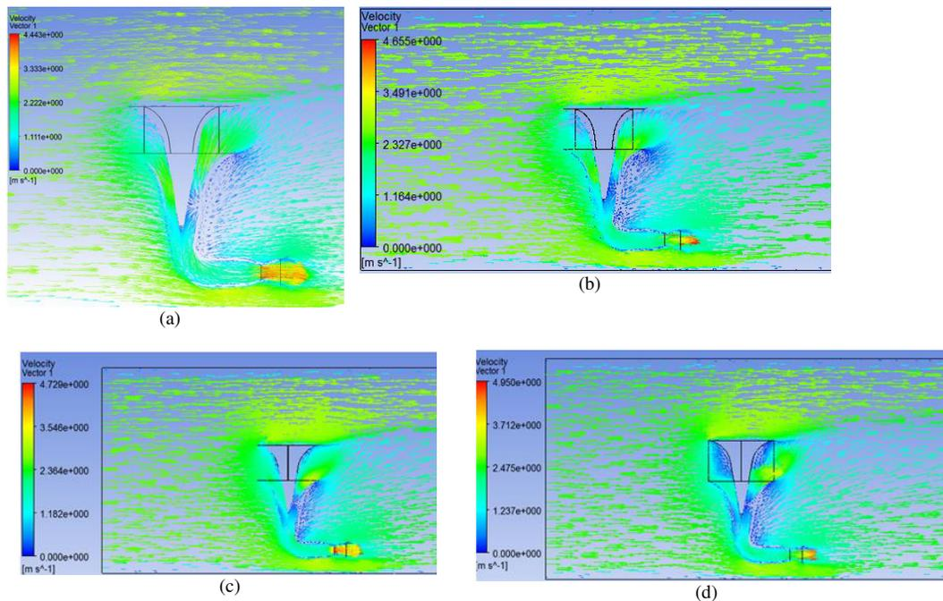
Figure 6. Velocity vectors of invelox duct with guide vane heights of a) 1.75 m, b) 2 m, c) 2.25 m, d) 2.5 m
