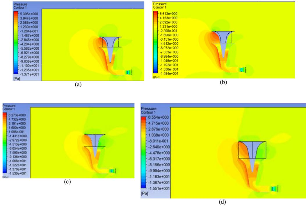
Figure 7. pressure contours of invelox duct with guide vane heights of a) 1.75 m, b) 2 m, c)2.25m, d) 2.5 m
