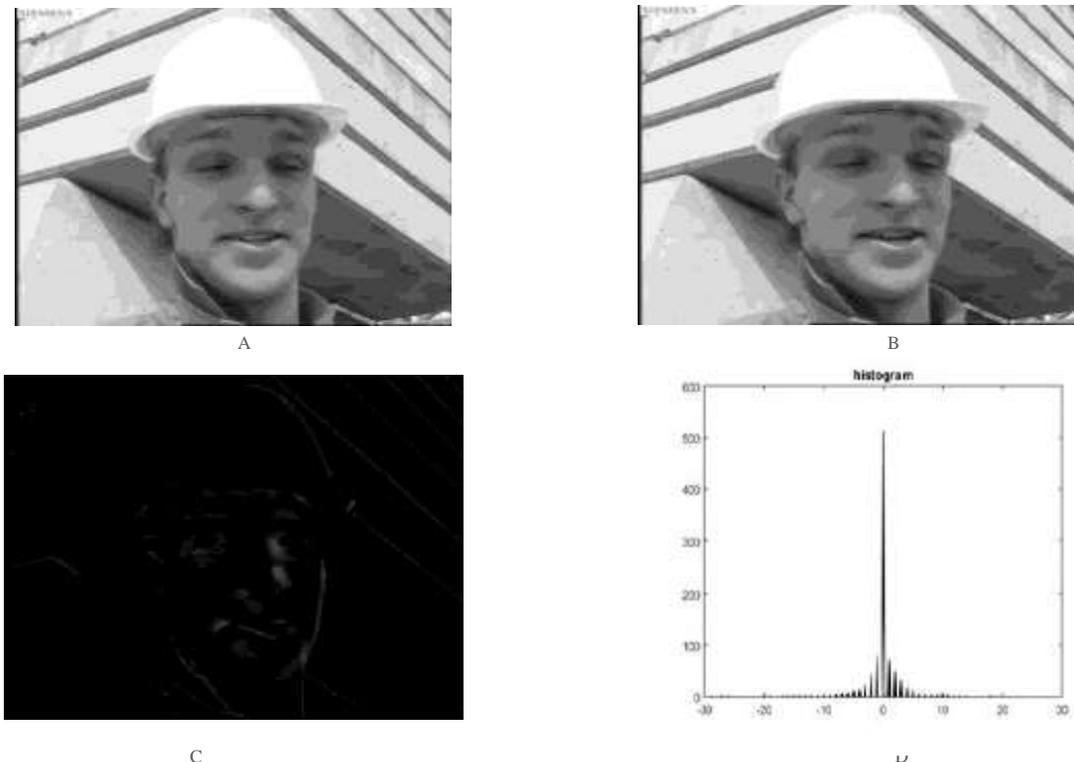
FIGURE 2 : AN EXAMPLE OF FRAME DIFFERENCING
