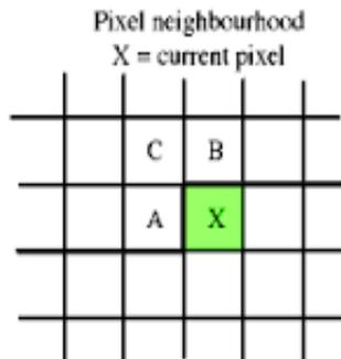
FIGURE 4 : THREE NEIGHBORING SAMPLES AROUND PIXEL X THAT NEEDS TO BE PREDICTED.
