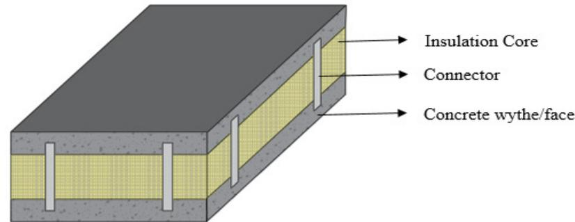
Figure 1. Elements in a sandwich panel.
