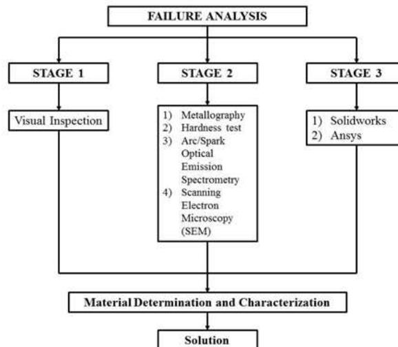
Figure 1. Methodology proposed for the failure analysis.
