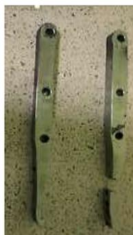
Figure 5. Failure of the clamping piece of the jaw.
