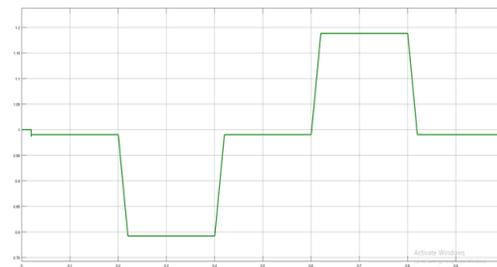
Fig-11:Source voltage and load voltage magnitude without PVA-UPQC (Voltage vs time)
