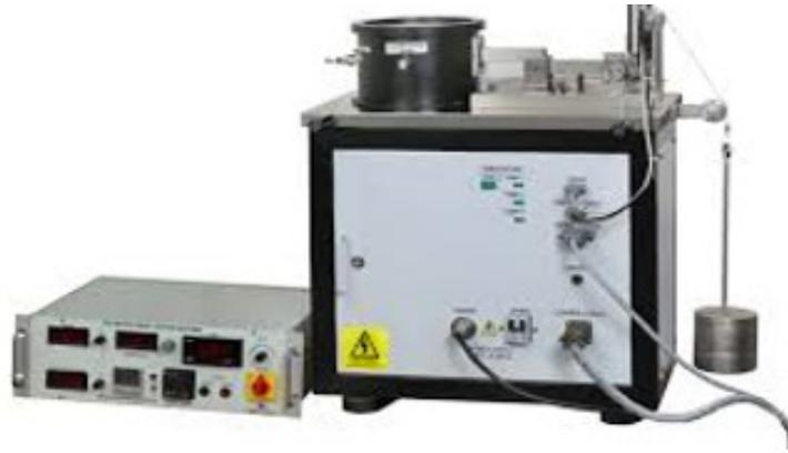
Figure.1: Pin on disc
