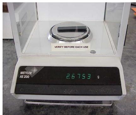
Figure.4: Mettler balance Electronic weighing machine
