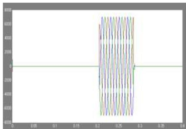
**Figure 6:** shows the injected voltage of DVR
