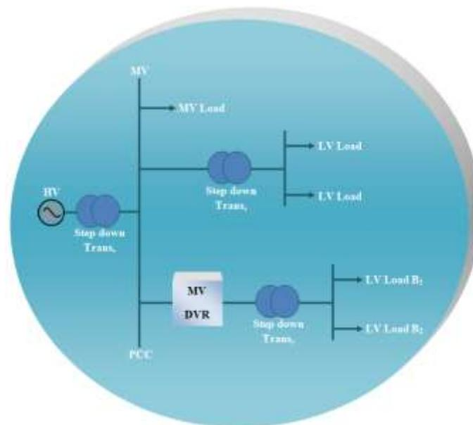
**Figure 2:** DVR join in a medium-voltage level electricity system
