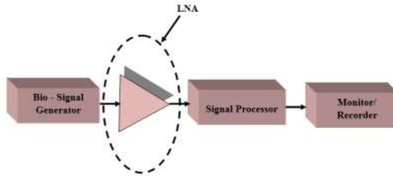
**Figure 1:** Block diagram of Bio-signal processing system
