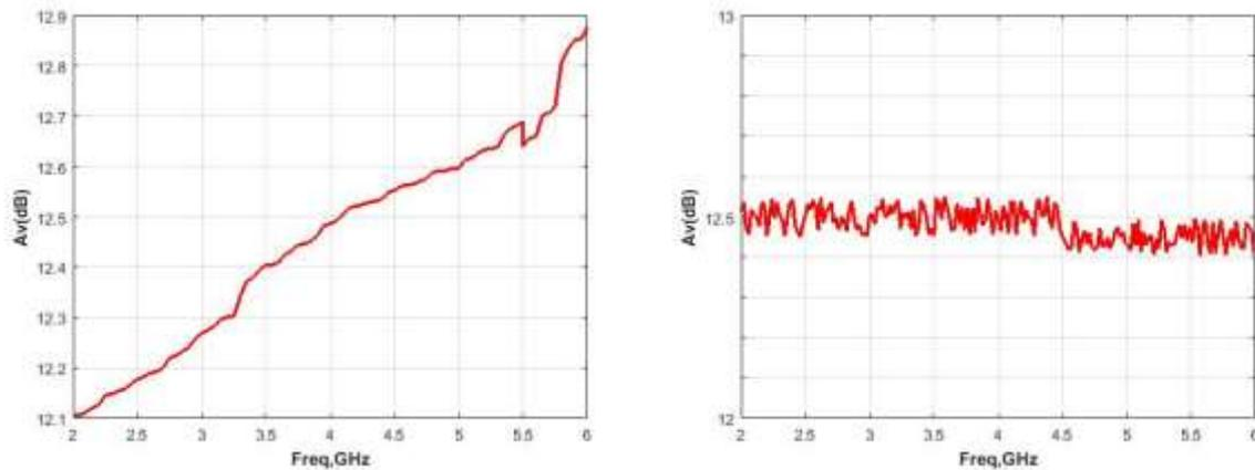
**Figure 5:**  $A_v$  (dB) in the present of parameter variations (a) without applying MSSO and (b) with applying MSSO
