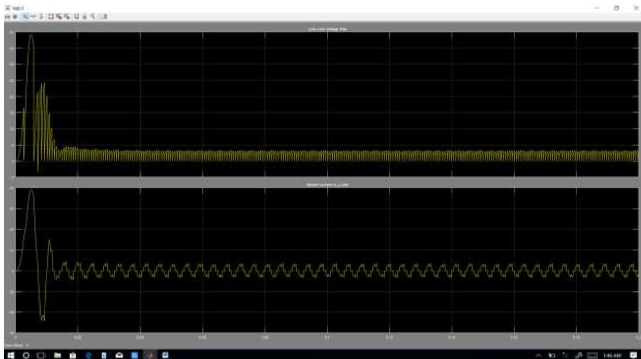
**Figure 4:** DC voltage and stator current of BLDC motor
