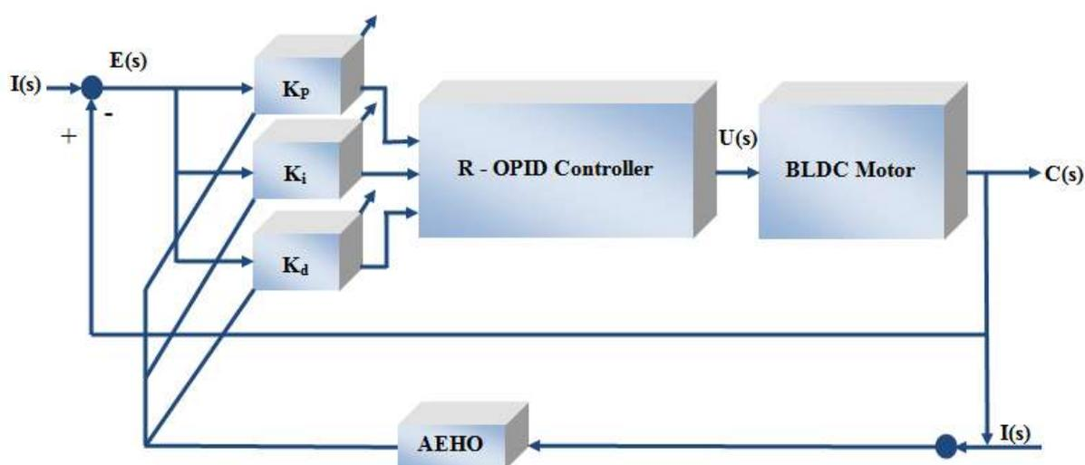
**Figure 1:** Block diagram for the proposed methodology
