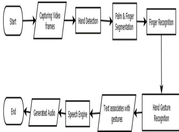
Fig. 2. Flow Diagram of Gesture to Audio
