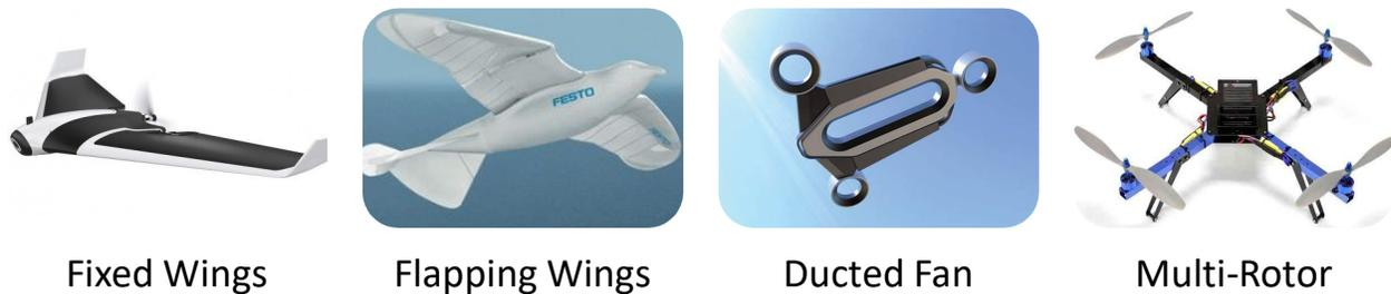
Fig 2: UAVs classified based on aerodynamics.
