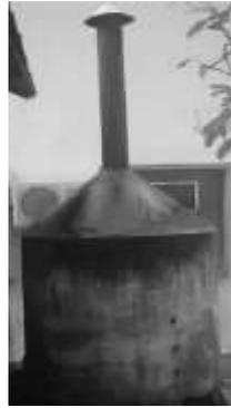
Figure1. Ferro-cement furnace
