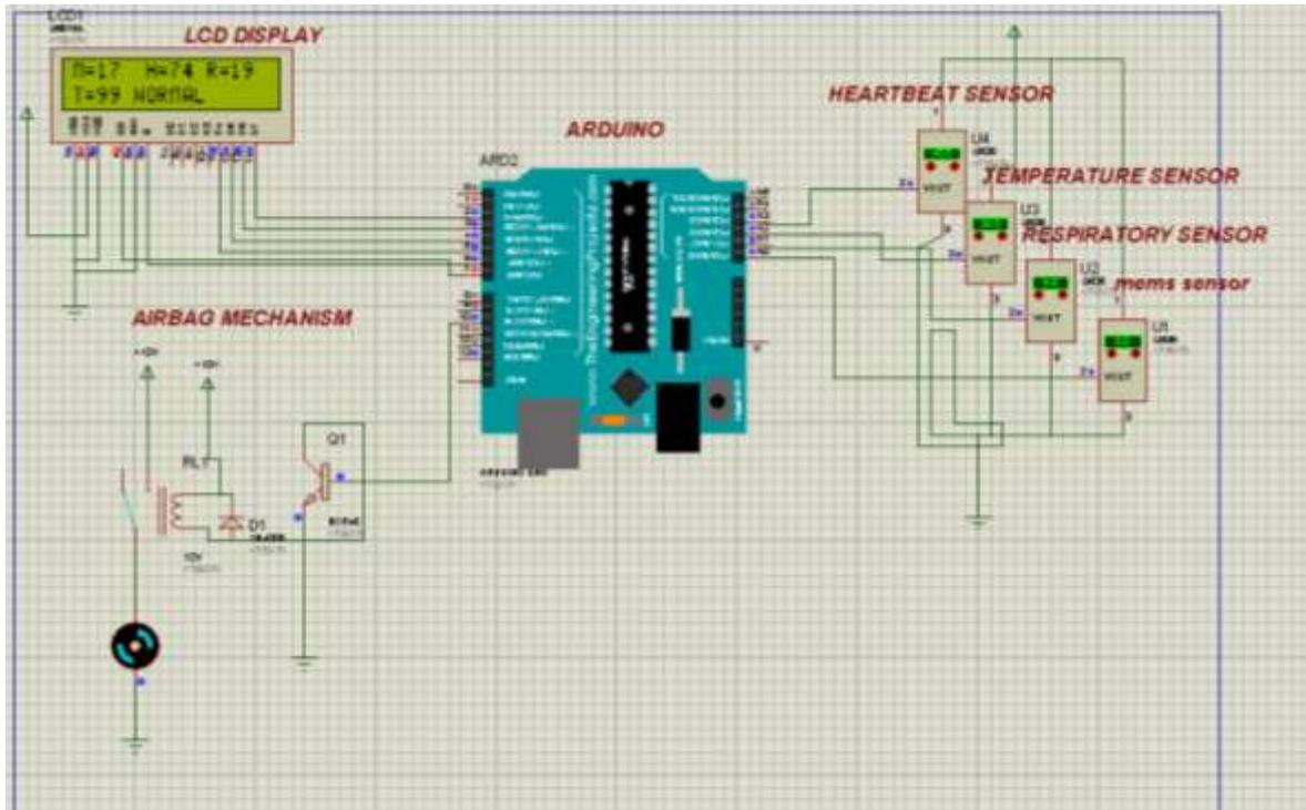
Figure 3. Simulation diagram of health monitoring of elder people under normal condition
