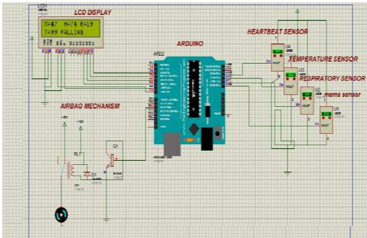
Figure 2. Simulation diagram of health monitoring of elder people under abnormal condition of MEMS sensor
