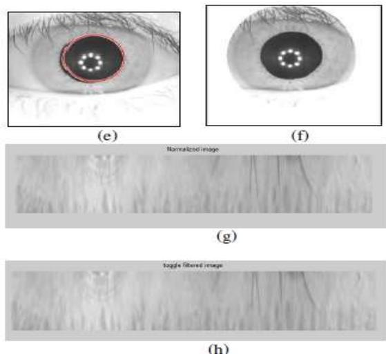
**Fig 5** Qualitative analysis CASIA database:(a) Input Image from CASIA database (b) Gaussian filter output (c) Gradient image (d) Canny Edge detection output (e) Pupil detection (f) Iris detection (g) Normalized image of **Daugman's** rubber sheet Model output (h) Toggle filter output
